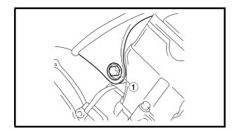
Pivot shaft wrench 90890-01471, YM-01471 Pivot shaft wrench adapter 90890-01476
