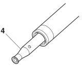
d. Install the oil flow stopper and inner tube bushing onto the inner tube "6".
