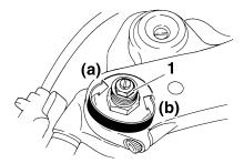
1. Spring preload adjusting bolt
