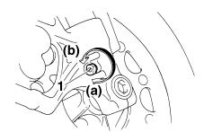
1. Compression damping force adjusting screw
