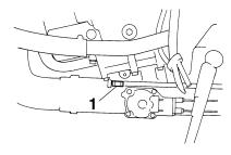
1. Engine oil drain bolt
