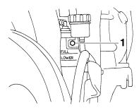
1. Brake fluid reservoir bracket bolt
