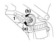
1. Compression damping force adjusting screw
