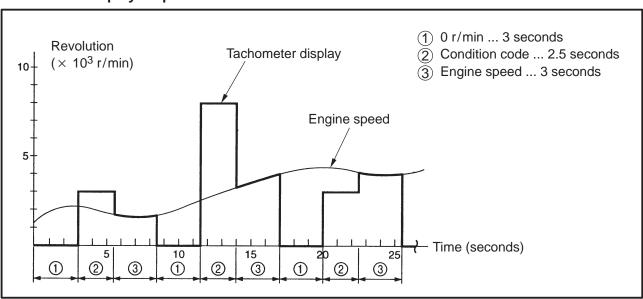
When more than one item is being monitored, the tachometer needle displays the condition codes in ascending order, cycling through the sequence repeatedly. If the engine is stopped, the engine speed ③ is 0 r/min.
