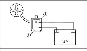
Does the radiator fan motor turn?
