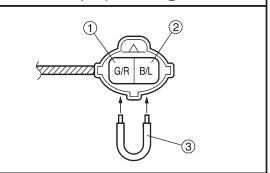
• Does the coolant temperature display "HI" and warning light comes on?
