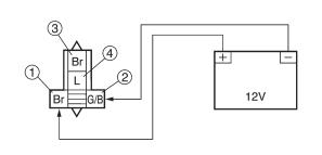
Does the radiator fan motor relay have continuity between brown and blue?
