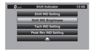
Select "Shift IND Brightness", then use the wheel switch to adjust the setting. Short push the wheel switch to confirm the setting and exit.
