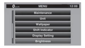
2. Select the desired brightness level by rotating the wheel switch, and then short push the wheel switch to fix the setting.
