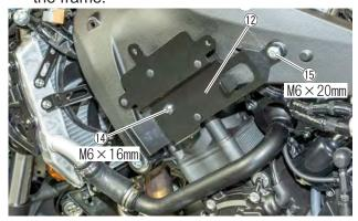
5. Install the ECU and BRKT., UPPER (1) using the BOLT, FLG 66 to the BRKT., UNDER 12.
