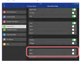
In the analog display mode, the voltage is indicated by level (0 to 5) by default. The display value can be changed according to the specification of the installed sensor. To change the display value, tap AIN Setting.
