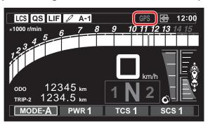
Since the GPS and oil-pressure warning icons are at the same location, the GPS icon does not light up when the the oil-pressure warning icon lights up (such as engine stop).
