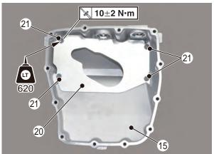
8. Attach (15) PAN,OIL to the engine by using (16)BOLT,BUTTON HEAD.
