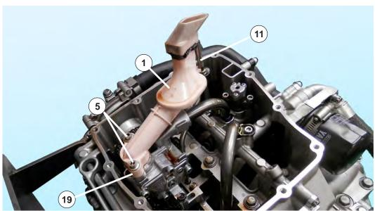
Fix (1) STRAINER HSG.ASSY., 11 PIPE, DELIVERY 1 and (23)BRKT.,STRAINER
