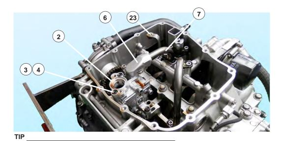
Visually confirm the condition of 6 PIPE,OIL 2 and 7 PIPE,OIL 1 periodically.
