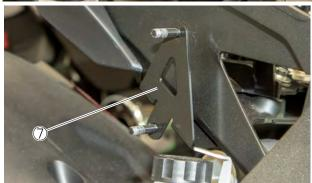
10. Install the rectifier/regulator to the BRKT.,REGULATOR 17 using the NUT,U FLANGE 10.
